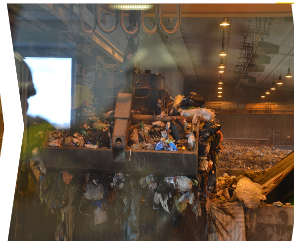
2. MATERIAL HANDLING WITH AUTOMATIC CRANE, WITHOUT NEEDING TO SEPARATE THE SECTORS
